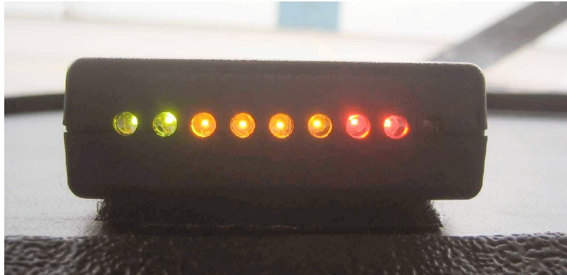
Figure 2-1. V-Speed ADS Mounted on Glare Shield in Horizontal Configuration
